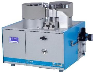
The new AM 04 Duomatic from Zoller + Fröhlich bridges the gap between fully automated and manual cable assembly. Its special feature is that two cross sections of any length can be processed at the same time. Operators can switch between set cross sections at the push of a button. A conversion process which used to take around two minutes and had to be undertaken by trained
